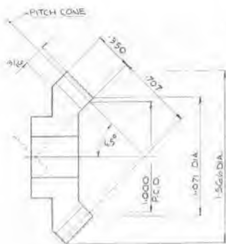
FIG 80 - A 20TOOTH 20DP PARALLEL DEPTH MITRE GEAR
